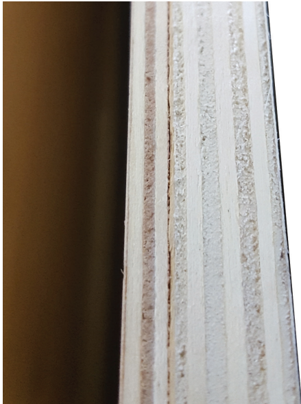
5/8" thick natural finish furniture grade plywood end panels
